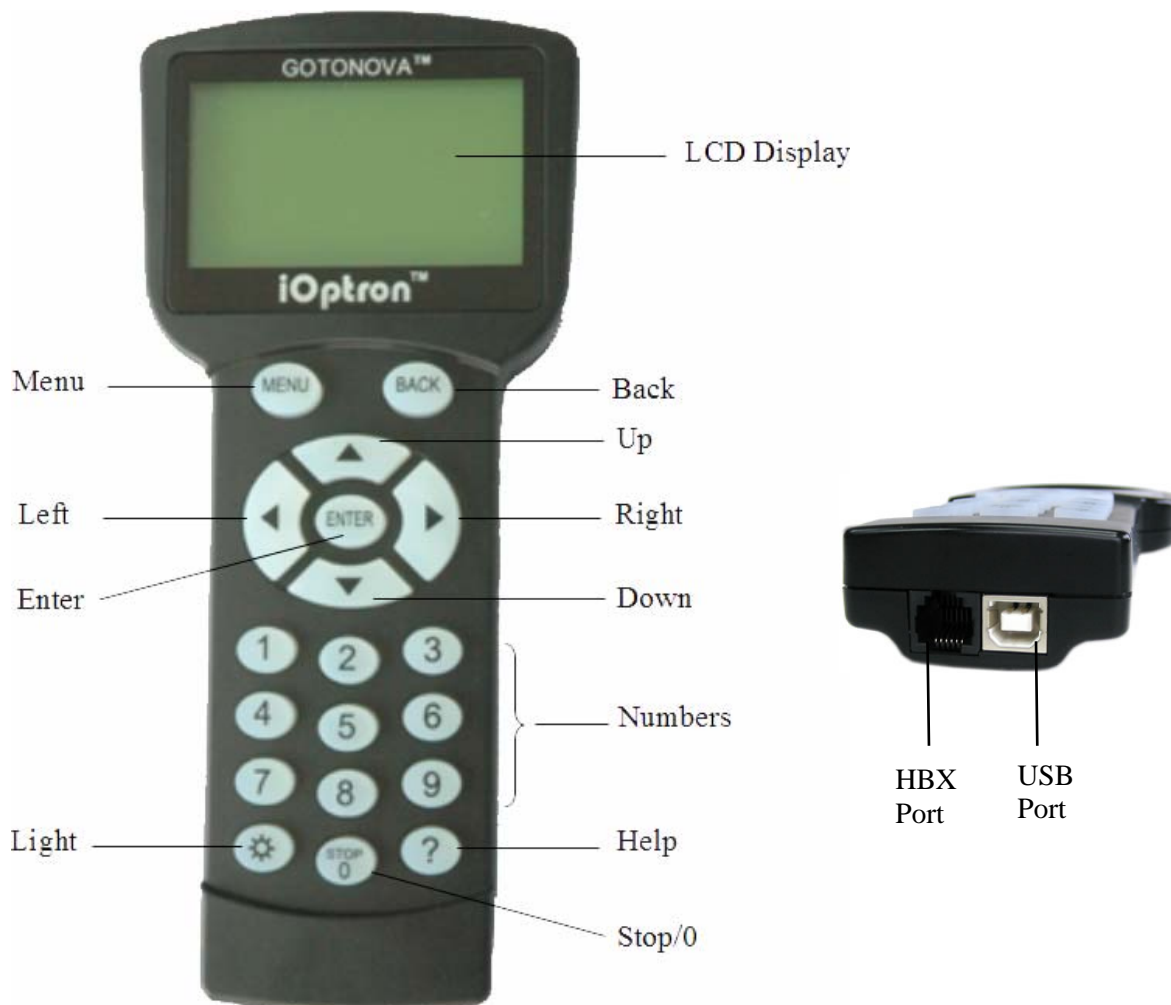
Figure 18. GoToNova 8401 Hand Controller
